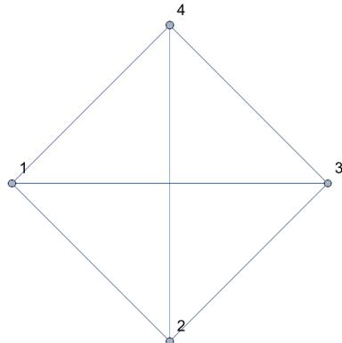
The example I made suggests that each pair of vertices is joined by an edge, i.e. it is a **complete** graph.
